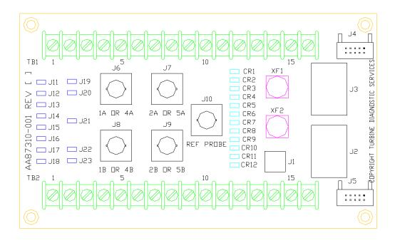
Below is a layout drawing of the REV A vibration termination board used to locate fuses, component and connections on the board.
